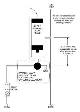
Figure 15-8 Typical Probe Installation
